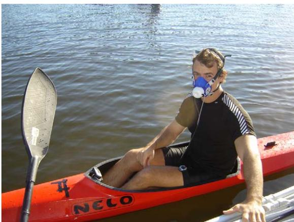
**Figure 7.** An example of the use of a portable metabolic assessment apparatus to measure exhaled gases. Note the global positioning unit taped to the kayak and the heart rate monitor on the left quadriceps.
